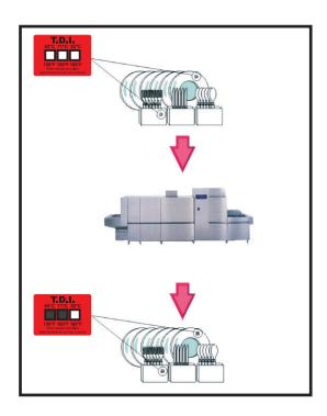
T.D.I's - An irreversible colour change from white/grey to black when standard dish washer (65°C), thermal/chemical disinfection (71°C) or thermal disinfection (82°C) temperatures have been reached.
